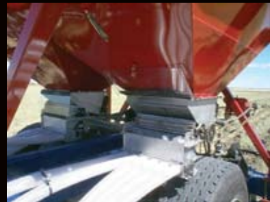
Stainless steel metering system delivers precise lbs/acre to 8, 12 or 16 rows
