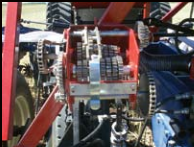
60 speed gearbox at 5% increments. Also available, hydraulic metering drive for variable rate application.
