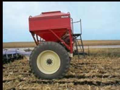
6 ton stainless steel hopper with rear platform and ladder.
