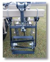
**Straight Blade Roller** Spring usage, best if used just prior to planting. Reduces clods and produces a firm seedbed.
