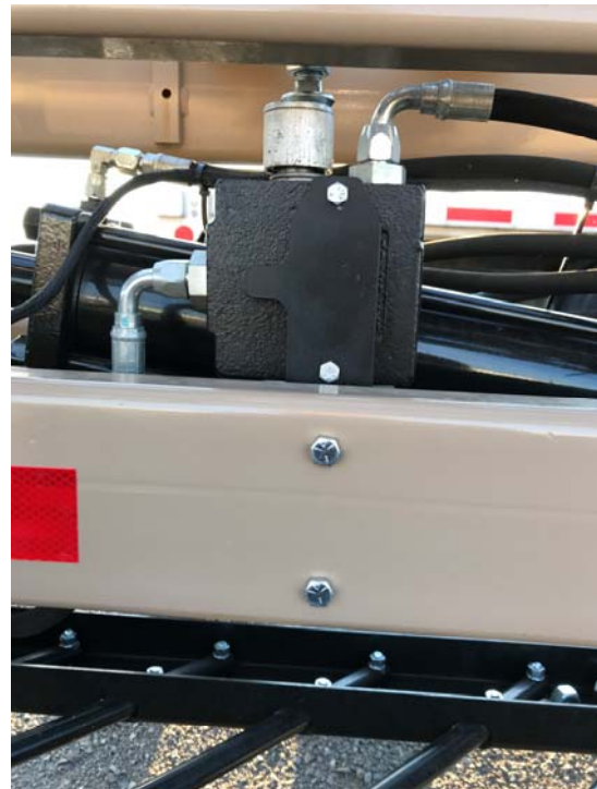
Stack Fold Valve mounted on rear frame of RF Cart near LH wing fold cylinder. (viewed from rear of cart)
