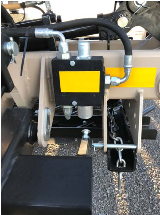
Wing Lock Valve mounted on front frame of RF Cart near LH axle ear. (viewed from front of cart)
